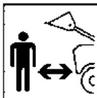
9. Ensure that the front loader is a safe distance away from overhead power lines.
